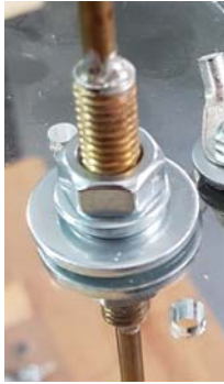
Fig. 7. Stiffener with washers and nuts
