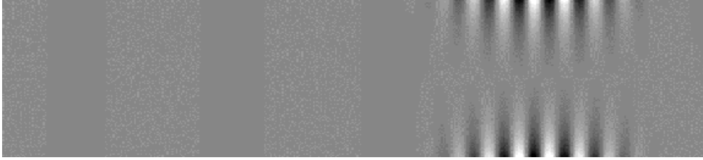
Fig. 5: Snapshot of the displacements amplitude (longitudinal component) at t = 267 \mu\text{s} : the A_0 mode is selected [17, 18].
