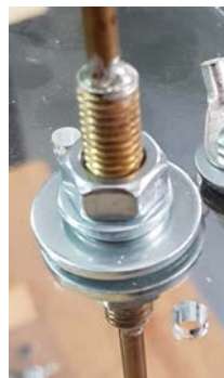
Fig. 9. Stiffener with washers and nuts.
